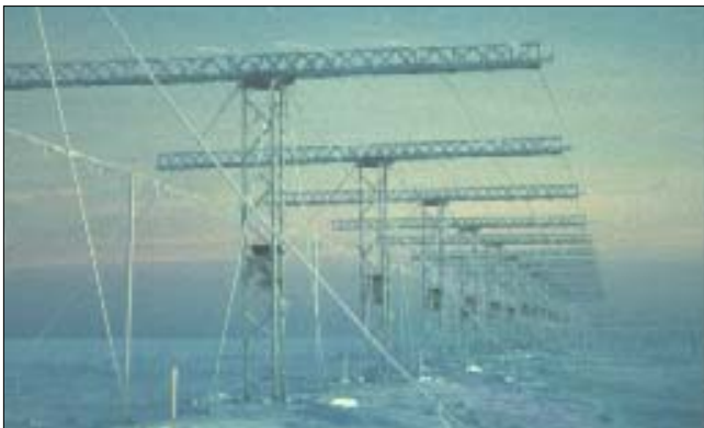
High frequency radar aerials at the BAS Halley Research Station used for investigating geospace
