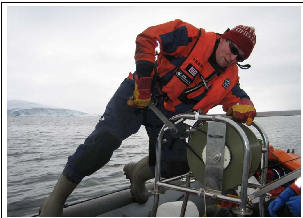
Hand winching the Niskin bottle to collect depth profile samples (Paul Mann)
