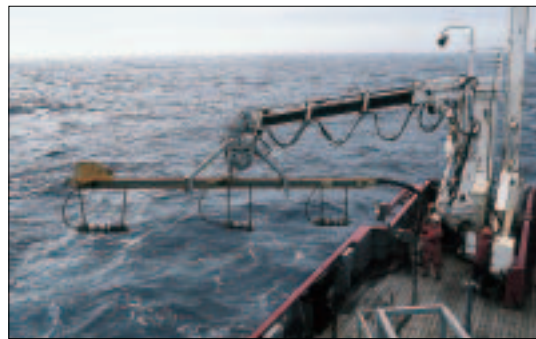
Air guns are deployed from the rear deck
