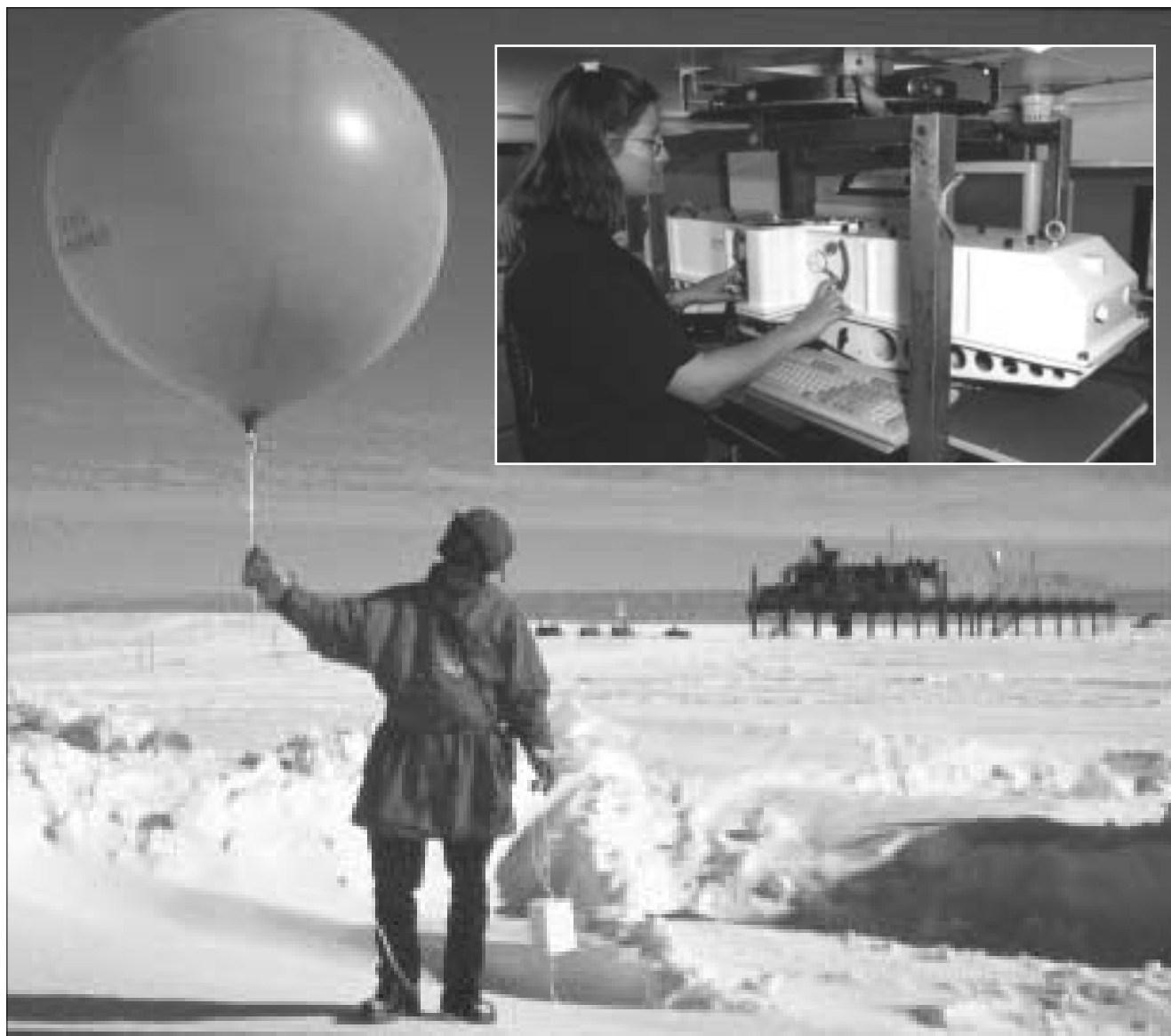
Balloon carrying a chemical radiosonde being released at Halley Research Station. Inset: A Dobson spectrophotometer in use at Halley
