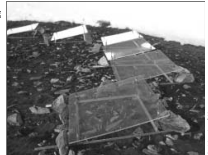
An experiment by BAS scientists using plexiglass to reduce ultraviolet light levels on Antarctic vegetation
