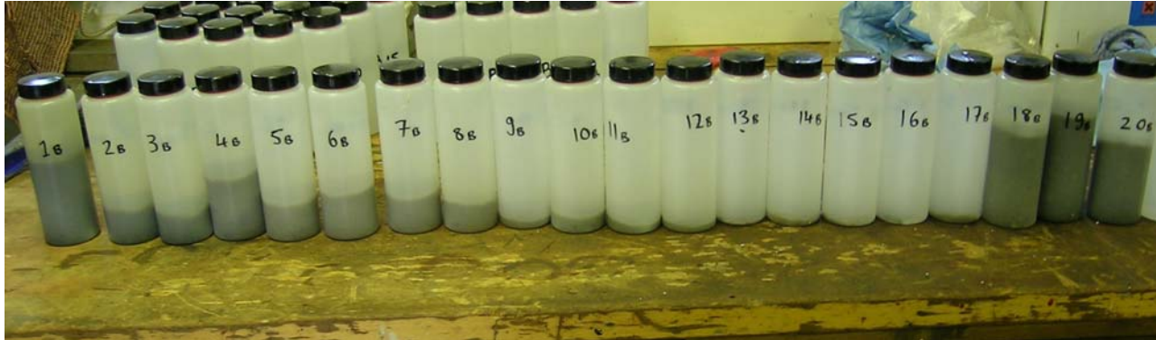
Fig. 2: Sediment trap sample collection bottles after surviving a year in the Antarctic coastal waters at the deep mooring site. Bottle 1B is sample collected throughout January 2005, Bottle 10B is October 2005, bottle 18B is ~January 2006 and bottle 20B is February 2006.
