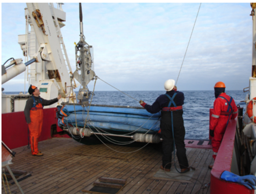
Figure 1. Deployment of the RMT8 trawl rigged with paired nets from the stern of the James Clark Ross. Due to the bad weather and various logistic constraints, the nets could only be deployed during daylight hours and were typically limited to depths greater than 20 m, which is considered suboptimal for sampling larval aggregations. Indeed, catch was extremely low for larvae, as well as for pelagic crustaceans such as krill and amphipods.
