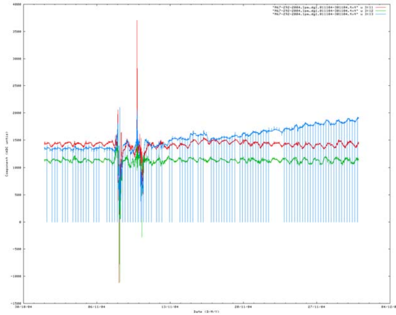
Figure 1. M67-292 raw X(red), Y(green), Z(blue) outputs in Nov 2004. Values before 4/11/04 have not been included in the released database.
